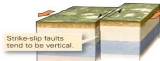
(d) On a strike-slip fault, one block slides laterally past another, so no vertical displacement takes place.
